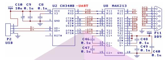
The image above use CH340T/CH340B (or CH340C) to realize USB to RS232 converter. CH340 provides common UART and MODEM signal, converts TTL to RS232 through level conversion chip U8. Port P11 is DB9 connector, the pin and its function are the same as common PC DB9 connector, the chips similar with U8 have MAX213/ADM213/SP213/MAX211 etc.
